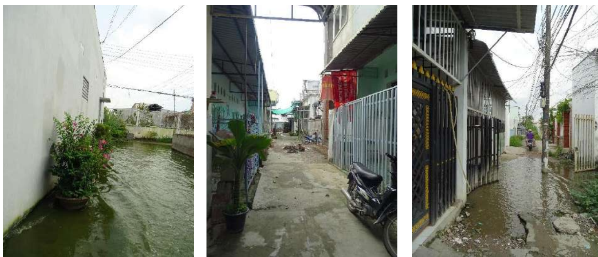
Fig. 5. Newly urbanized areas in Can Tho. Most unused parcels are covered with concrete, and houses have not been elevated. Photos by the author
